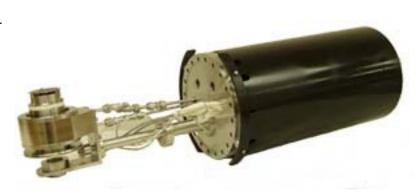
Rotating heater shown in deposition position with multi-target manipulator.
